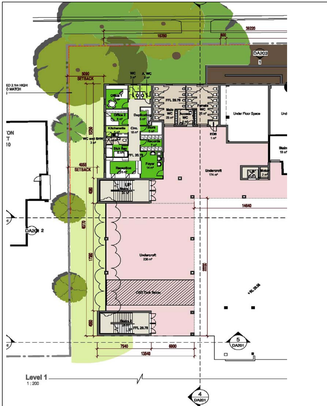
Figure 6: Detail of the revised plan Issue C above shows the undercroft area enclosed with an acoustic wall to shield noise to the adjoining residential flat building. The amendments were accompanied with an acoustic report assessing noise impacts to adjoining property. This has been assessed by Councils Health (Acoustic) Officer and found to be satisfactory subject to standard conditions.
