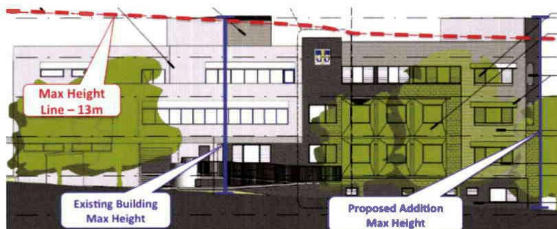
Figure 5: Elevations outlining the encroachments to the maximum height control. The dotted red line across the top of the building represents the 13m height control.
